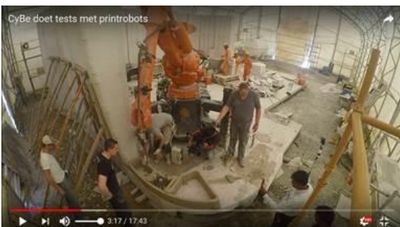
Person in grey t-shirt removing excess material due to tilting of print head
