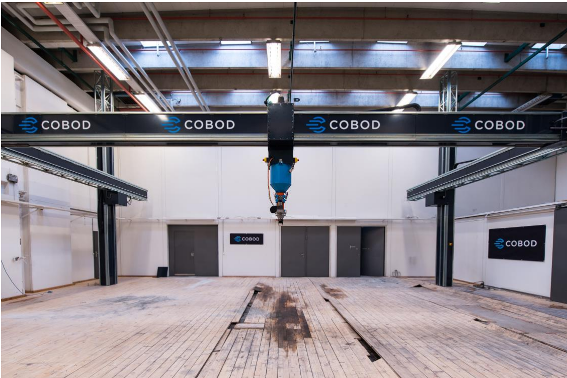
Picture of a BOD2 3D construction printer when being tested before shipment.
